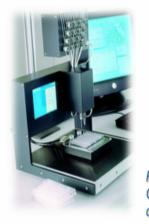
Fully-automated Oocyte two-voltage clamp system
